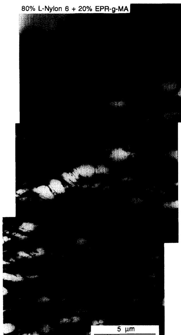
**Figure 18** TEM photomicrograph showing the morphology of the deformed zone in the vicinity of the arrested crack for the L-Nylon 6/EPR-g-MA blend
